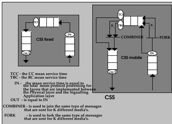
Figure 5: Queuing network of the CSS for B-ISDN-to-the-CSS.
