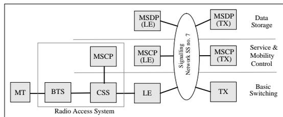
Figure 2: Overview of basic UMTS architecture.
