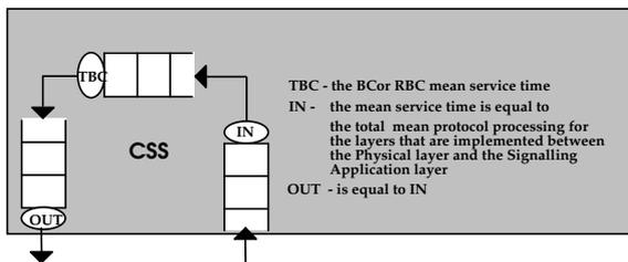
Figure 6: Queuing network of the CSS for B-ISDN-to-the-MT.
